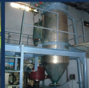
Agitated Flash Dryer [ Options of various designs of Attritors ]
