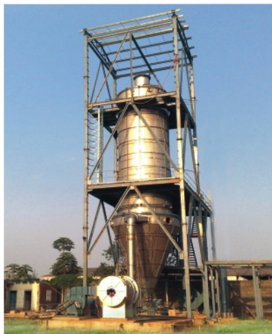
SINGLE-FLUID NOZZLE, CO-CURRENT MODE
