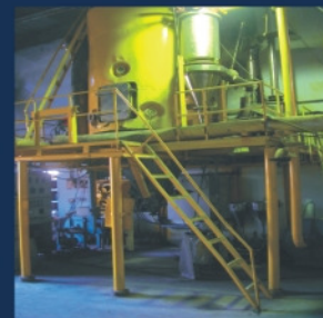
Multistage spray dryer [ Various design of atomizer wheels ] Vibratory fluid bed dryer
